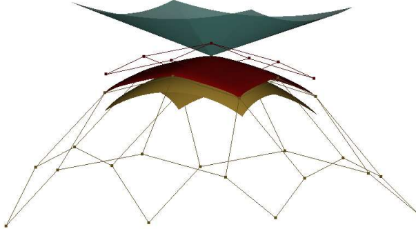
Figure 2: The original surface (below) and the interpolating linear blending surface. The permissible positions of the upmost control point is shown by a volume bounded by a cone-like surface.
